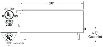
Gas: 3/4" NPT rear gas connection, specify type of gas and altitude if over 2,000 feet.
